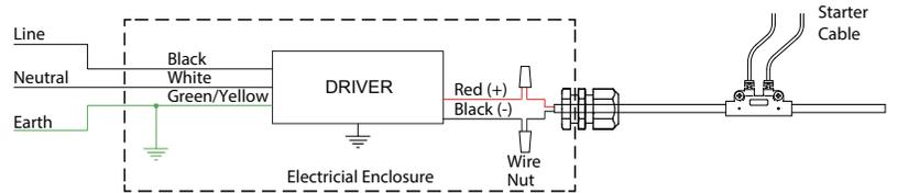
5. Connect the AC earth wire to the ground stud inside the driver enclosure.
